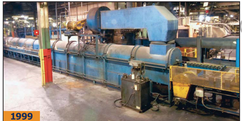
GRANCO CLARK 60' natural gas fired automatic pass-through billet preheat furnace
